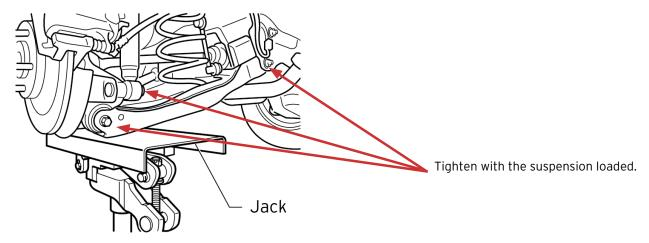
Tightening suspension components unloaded may cause:
